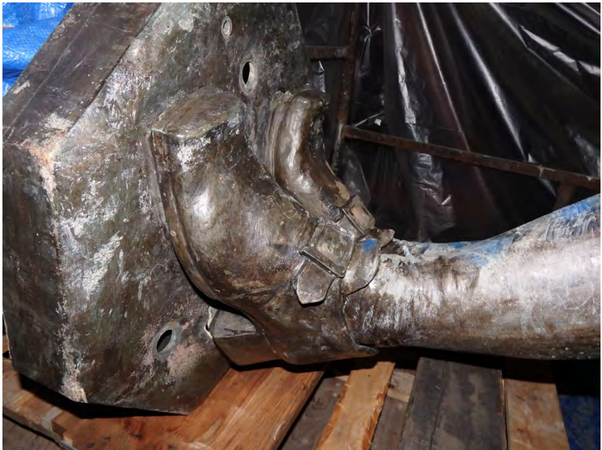
Tear in bronze under the left heel and bent base.
